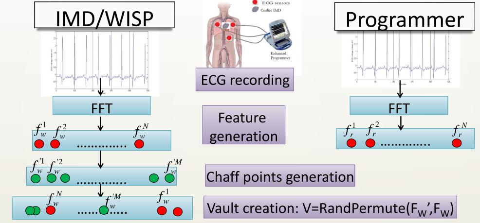
To be authenticated to the IMD, the programmer should identify the vector I of common features positions during generation
