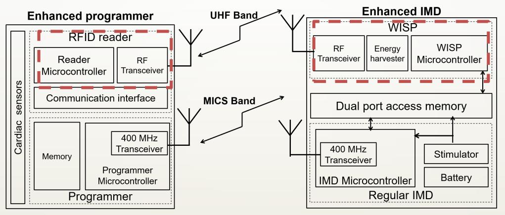
Integration of RFID system to implement an energy harvesting solution
